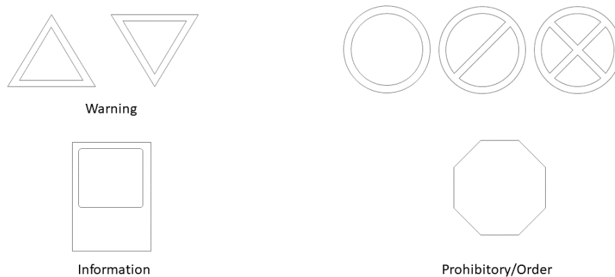
Fig. 4.2. Commonly used shapes for Road Signs.
